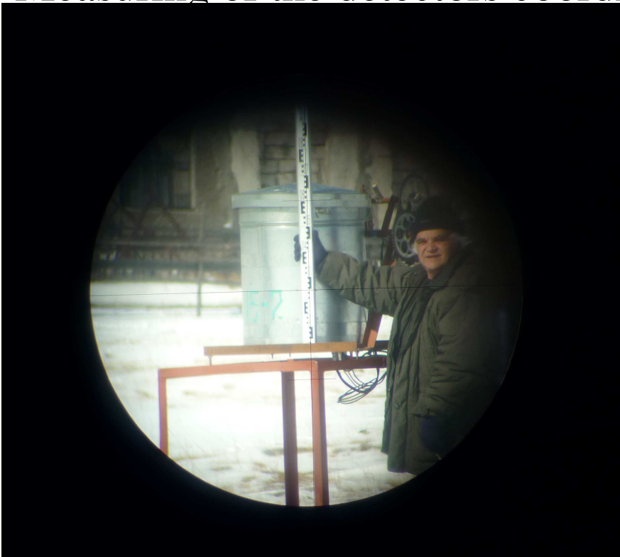
Measuring of the detectors coordinates (x,y,z) – accuracy ~ 10 cm.
