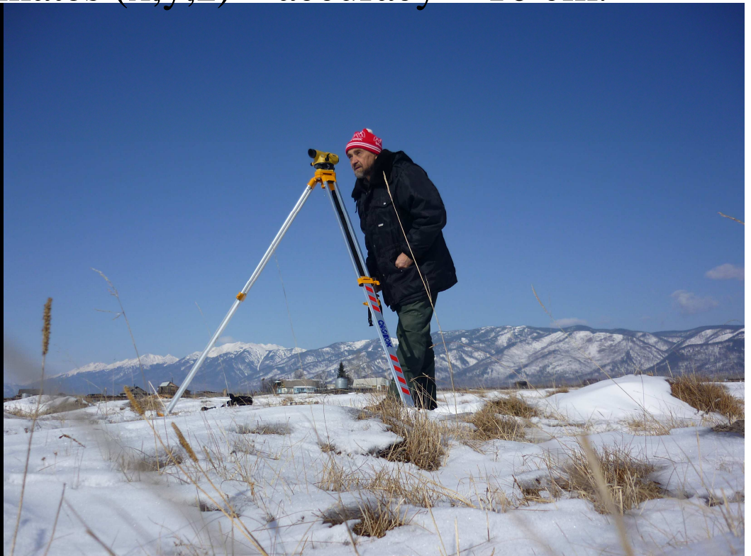
Measuring of the detectors coordinates (x,y,z) – accuracy ~ 10 cm.
